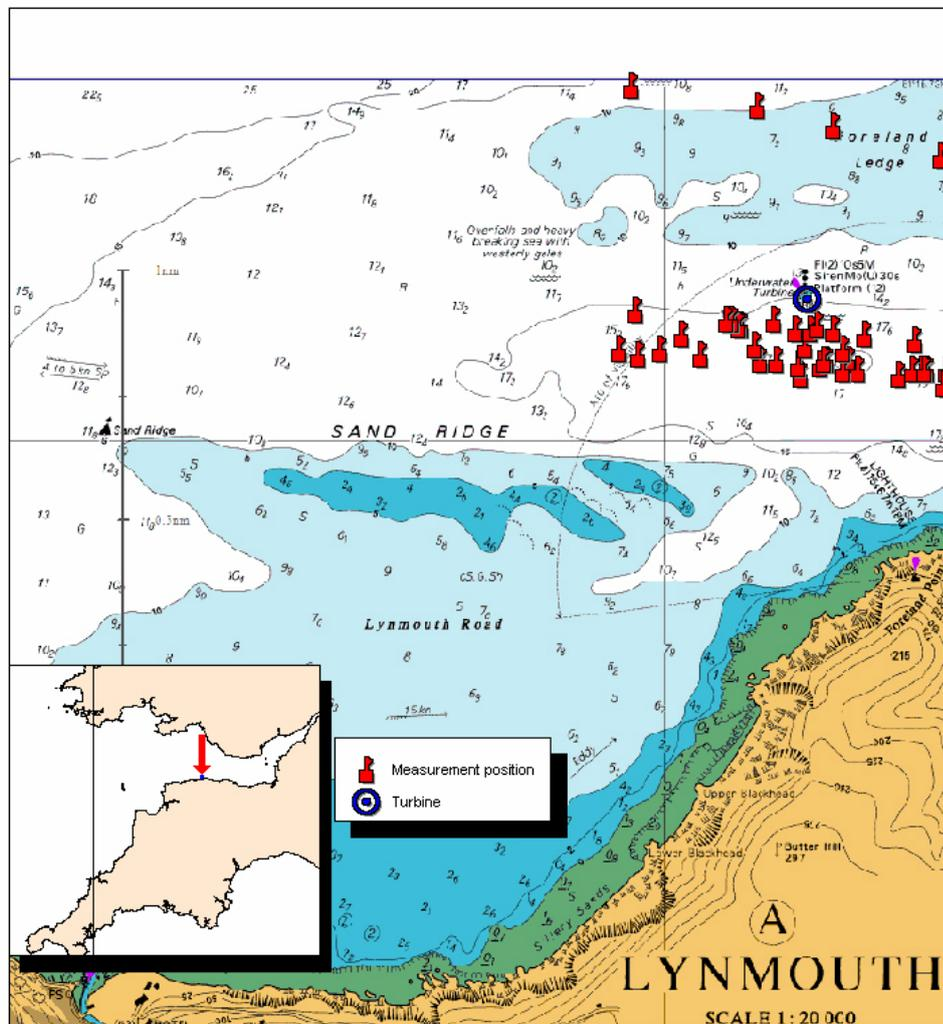
Figure 7-1: Chart showing the positions of the MCT tidal current turbine in the Bristol Channel, and the positions of the underwater noise measurements on 9<sup>th</sup> March 2005 (source material: UK Hydrographic Office)
