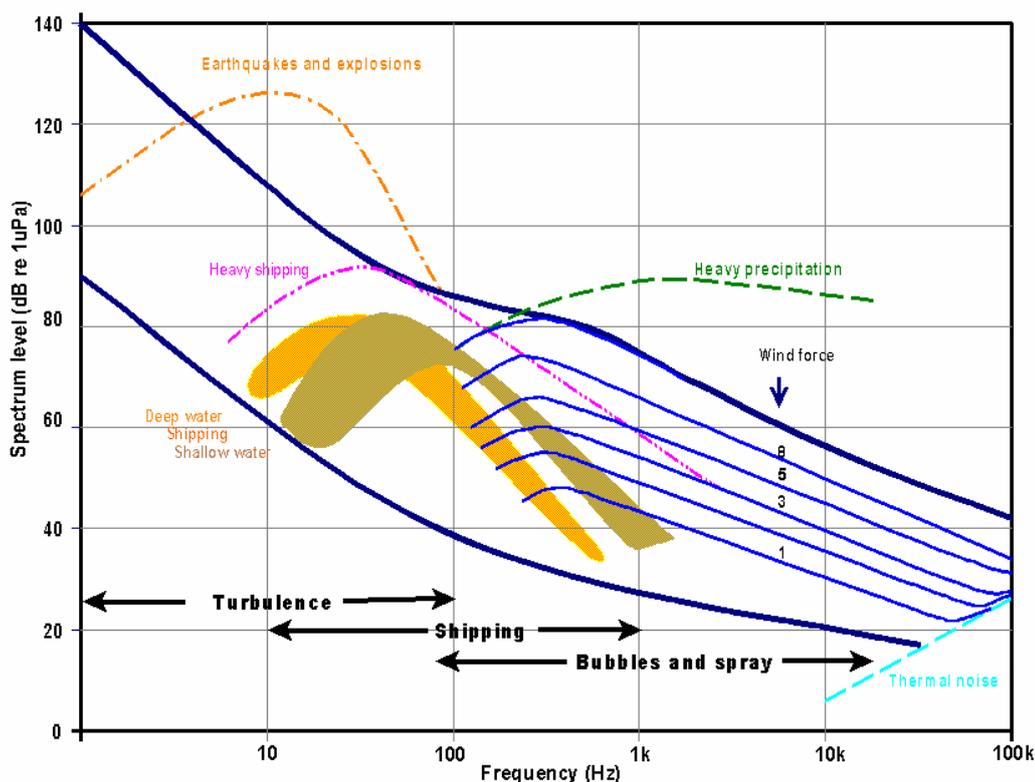
Figure 2-3: Composite of ambient noise spectra. (Adapted from [3])
