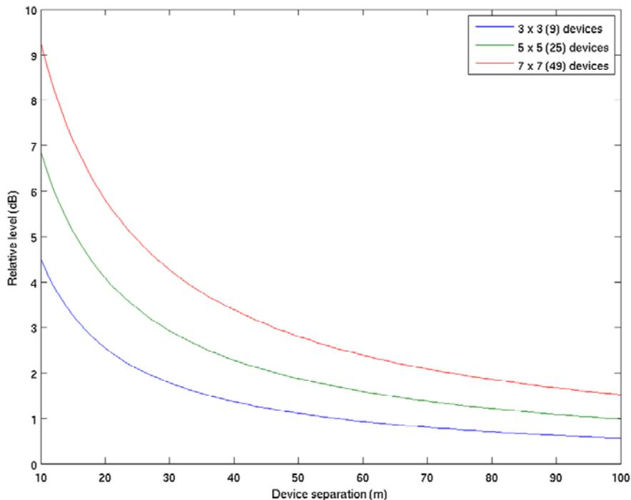
Figure 8-8: Noise level relative to the noise of a single device, at the centre device of a square array, as a function of the separation between devices
