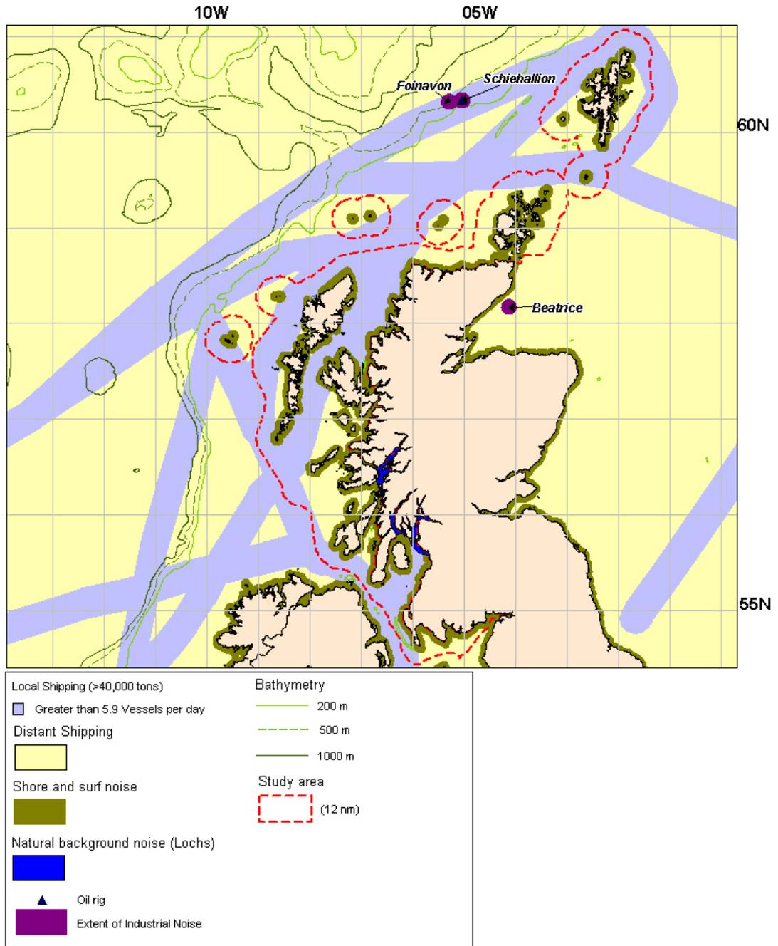
Figure 5-1: Dominant noise sources in the SEA study area when there is little or no wind and precipitation. When weather conditions deteriorate wind and precipitation noise will dominate over most of the area and the region in which shore and surf noise dominates will extend further offshore.
