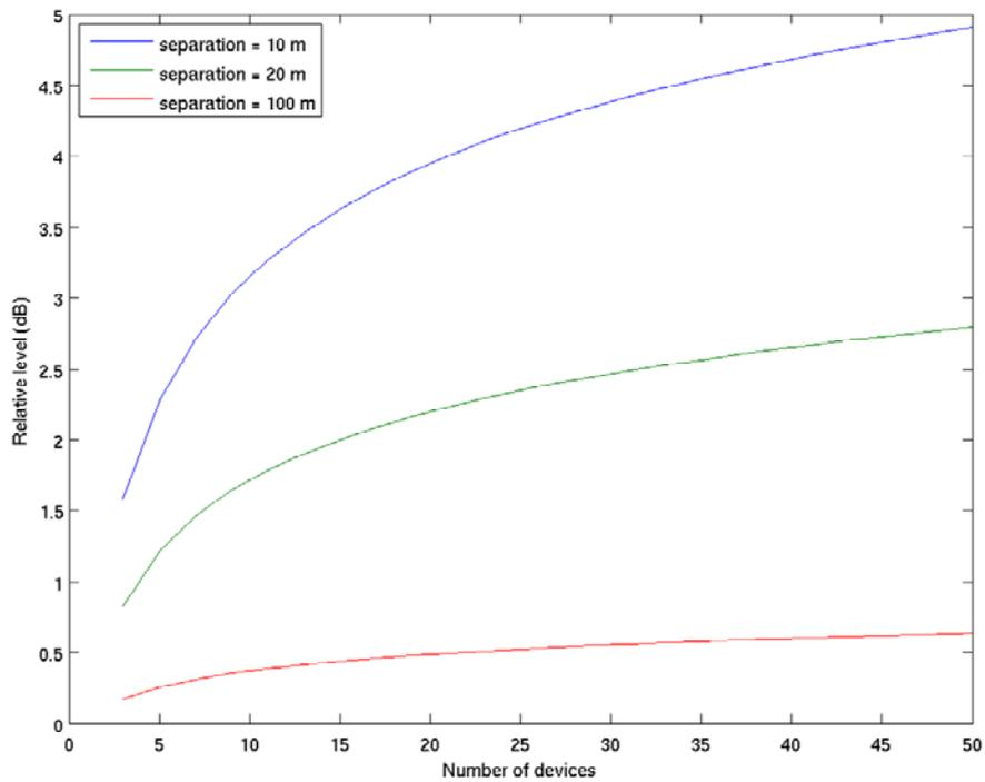
Figure 8-7: Noise level relative to the noise of a single device, at the centre device of a linear array, as a function of the number of devices in the array
