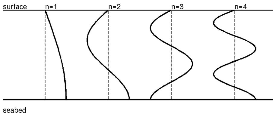
Figure 2-2: Sound pressure versus depth for the first four normal modes, for a pressure-release surface and a rigid bottom (adapted from [2])
