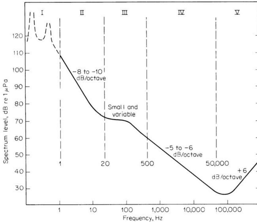
Figure 2-1: Deep water ambient noise (adapted from [2])
