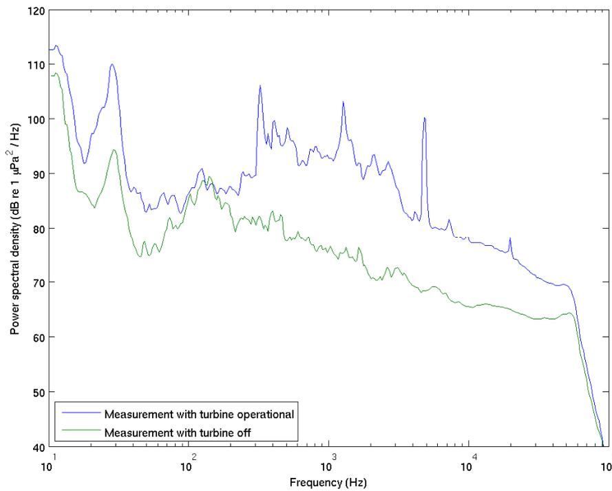
Figure 7-3: 1/27<sup>th</sup> octave spectra of ambient noise and turbine noise at the Lynmouth site (data courtesy of MCT and Subacoustech Ltd)
