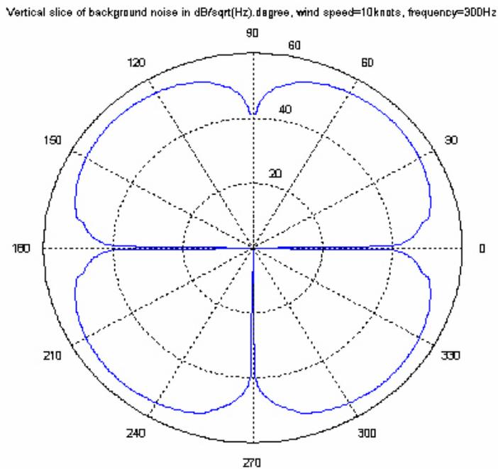
Figure 8-4: Vertical directionality (level v angle) of ambient noise for an olivine bottom
